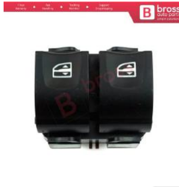
BDP1095 Window Regulator Driver Door Switch 254113300R For Renault Captur Clio 4 Zoe Dacia Duster Lodgy
