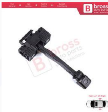
BDP1399 Rear Door Stop Check Assy Limiter Strap for BMW 1 Series F20 F20N 2011-2019 5-Door 51227446727
