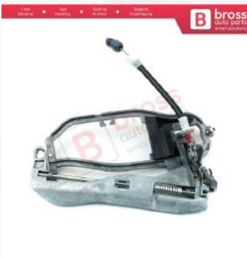
BDP173 Car Door Handle Housing Carrier Bracket Housing Front Left 51218243615 For BMW X5 E53 2000-2006
