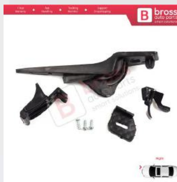
BHL557 Headlight Holder Mount Repair Bracket Tab Set Right Side for Ford Fiesta B299 B409 B479 2013-2019 D2BZ13008L
