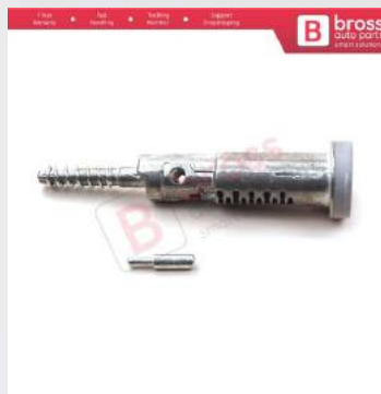
BSP638 Ignition HU46 Lock Cylinder Shaft For Opel Astra
