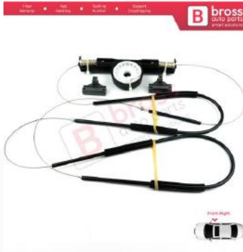
BWR5431 Power Window Regulator Repair Set Front Right Door for Ford Mondeo MK3 B4Y BWY B5Y 2000-2007 4/5 Door 1S71F23200AB
