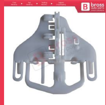
BWR5355 Power Window Regulator Repair Clips Front Right for Dodge Nitro 2006-2012 Jeep Liberty KK 2008-2012 68004820AA
