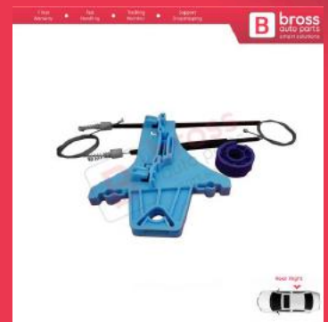
BWR5061 Window Regulator Repair Kit Rear Right for VW Polo Vento MK5 6R 6C 61 2009- 2022 4/5 Door 6R4839462
