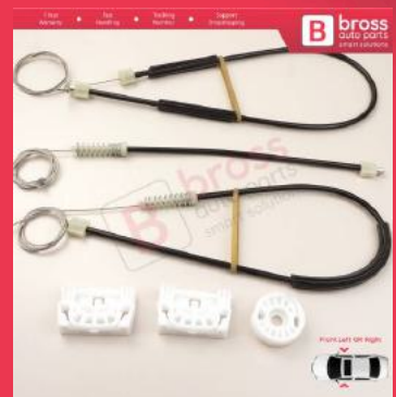
BWR5230 Window Regulator Repair Set Front Left or Right Door for Mercedes Vito Viano Mixto V Class MK2 W639 2011-2014 6397200446 6397200546
