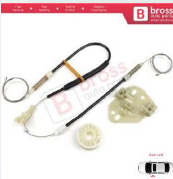
BWR1014 Window Regulator Repair Kit Left Door for Mercedes Axor 2001-2005 Atego MK1 1998-2004 9737200346
