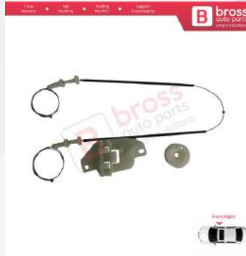
BWR5242 Power Window Regulator Repair Kit Front Right for Hyundai Starex H-1 Grand MK2 TQ 2007-2024 824044H010
