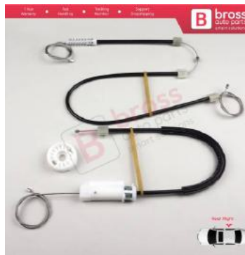
BWR973 Window Regulator Repair Kit Rear Right for Mercedes CLS Class C219 W219 2004-2011 A2197300846
