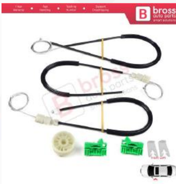
BWR266 Window Regulator Repair Kit Front Left Door for Renault Laguna MK2 X74 BG0/1 KG0/1 2001-2008 8200000937
