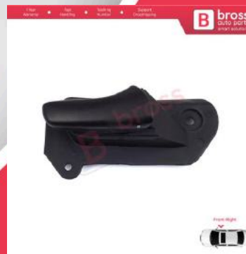
BDP1422-2 Front Right Interior Door Handle Opener Black for Vauxhall Opel Astra F MK3 T91 T92 1991-2001 90430130
