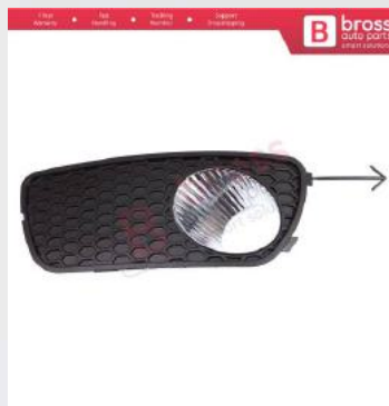
BSP1187-1 Front Bumper Fog Light Frame Housing Left for Fiat Palio Siena MK1 178 2007-2016 Albea 2002-2012 51703147
