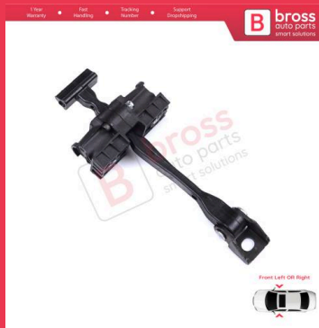
BDP1407 Front Door Stop Check Assy Limiter Strap for BMW 2 Series MK1 F45 F46 Tourer 2013-2021 51217404897
